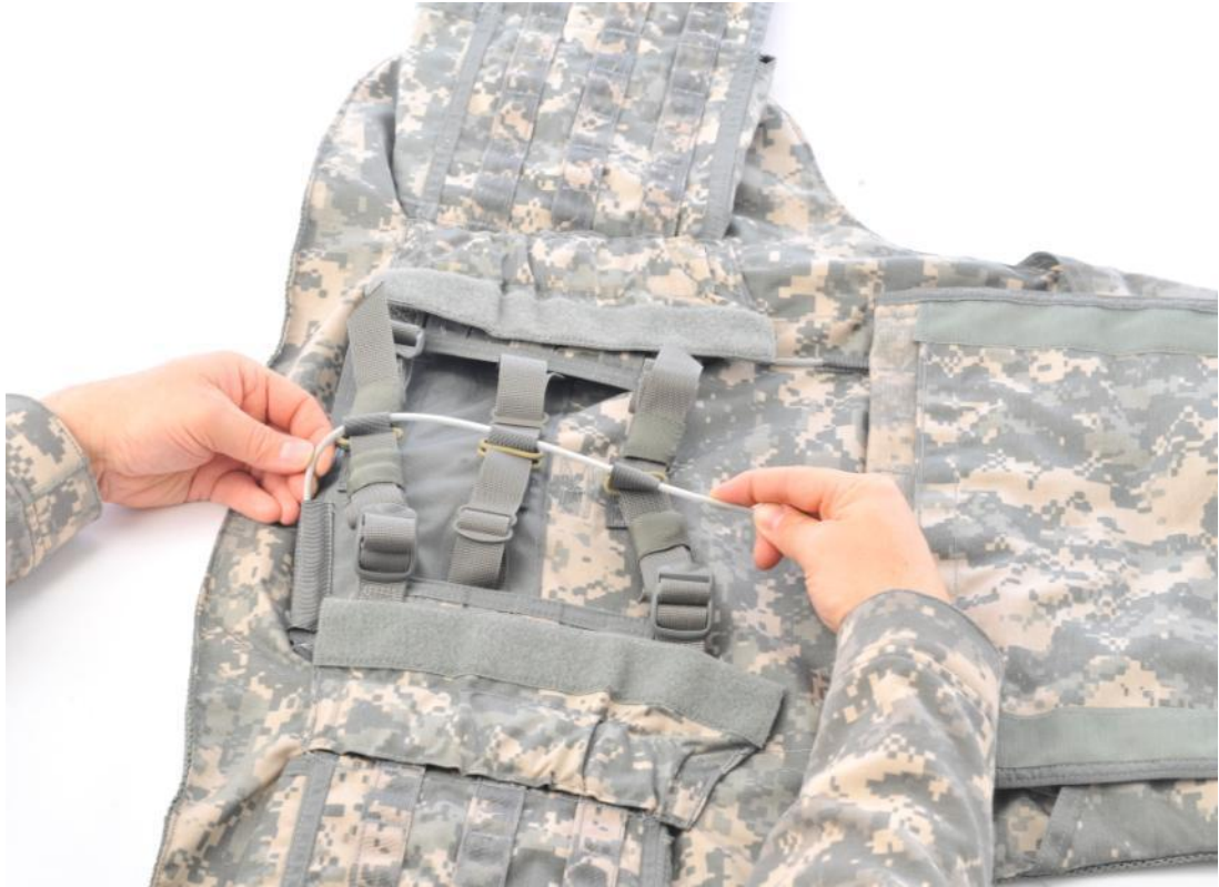
Figure D-3.20. Routing Long Cable.
