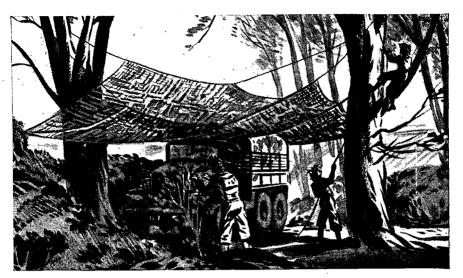
FIGURE 47.—An overhead screen provides good concealment. It is particularly valuable over more permanent parking places because it allows considerable freedom of movement underneath it and because vehicles can come and go while the camouflage remains in place. With this type of cover, a tight flat screen is unnecessary.
