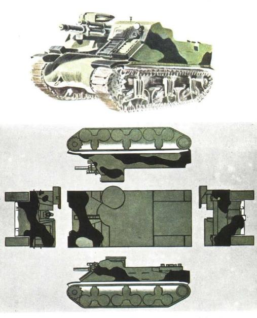
FIGURE 38 ① and ②.—Ground view and pattern plan of tank destroyer painted olive drab and black, the undersurfaces countershaded white. Keep patterns bold and simple.
