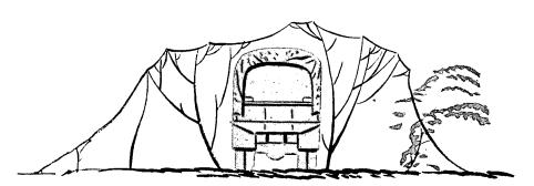
FIGURE 46 ①.—Nets must be propped above and away from a vehicle so that a distorted outline is formed. Branches or poles are used for this purpose. To eliminate shadow, extend net at a gradual slope from center of object covered.
