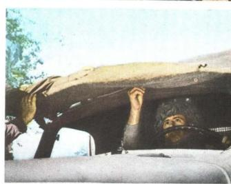
FIGURE 22. — Mud and leaves applied liberally to the windshield reduce shine. When moving, the area traversed by the windshield wiper should remain clear.
