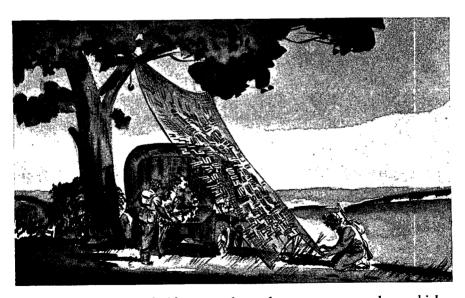
FIGURE 48.—A sloped side screen hung from a tree conceals a vehicle from oblique observation. Repairs, unloading, and other activities can be carried on behind it. Camouflage nets used as drapes can often combine the principles shown in figures 47 and 48, and thus provide concealment from both ground and air observation.
