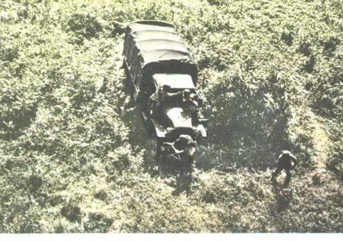
FIGURE 49 (a) and (b).—Steps in the erection of a drape. In upper picture, truck is parked close to bush. Reflecting surfaces which may shine are covered before the net is put on. Rear curtain is dropped to cover shadow in cargo space. In lower picture, net is unfolded so its long axis is diagonally over the truck and slightly off center.
