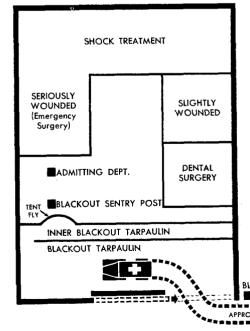
FIGURE 85.—Diagram of blackout system for medical clearing station as laid out in warehouse. Door openings must have effective blackout flaps, since wounded will be brought in and out frequently.
