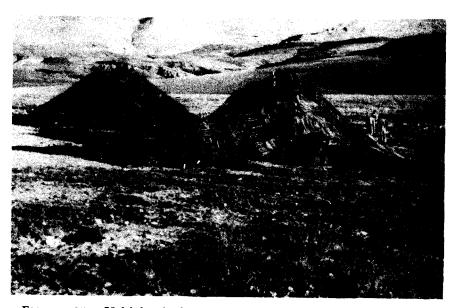
FIGURE 20.—Vehicles in barren terrain. Drapes made of garnished twine nets transform these rectangular shapes into mounds.
