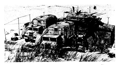
FIGURE 52 ① and ②.—Drapes, placed to resemble surrounding terrain, cover headquarters in desert. Note compact assembly of vehicles under framework being erected to simulate mound shown below. Installation is effective against both direct and photographic observation. This is a necessary exception to dispersion; vehicles are dispersed by groups rather than by individual vehicles.
