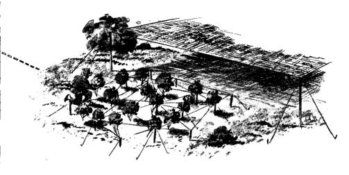
FIGURE 62 (4).—Blast marks can be concealed. One method of camouflaging blast marks is to cover area with network of wire supported on 2½-ft. stakes. This network is used to support branches and other suitable foliage in natural position over blast mark area. The network should be irregular in outline and cover a larger area than the blast mark.
