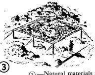
(3).—Natural materials must be replaced as soon as they show signs of withering. Foliage must be cut and disposed of where it will not attract attention. A decoy position is a solution to the disposal problem.
