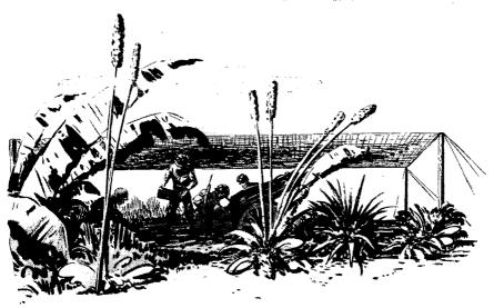
FIGURE 69.—When there is no natural cover, net may be used for flat-top to cover position. See FM 5-20, Camouflage, Basic Principles, for erection procedure of small flat-tops.
