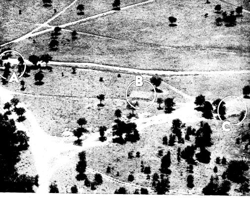
FIGURE 19.—Portion of 155-mm howitzer battery showing effect of tying in flat-tops with existing scattered trees **A** and **C**. **B** shows conspicuousness of position in open terrain.
