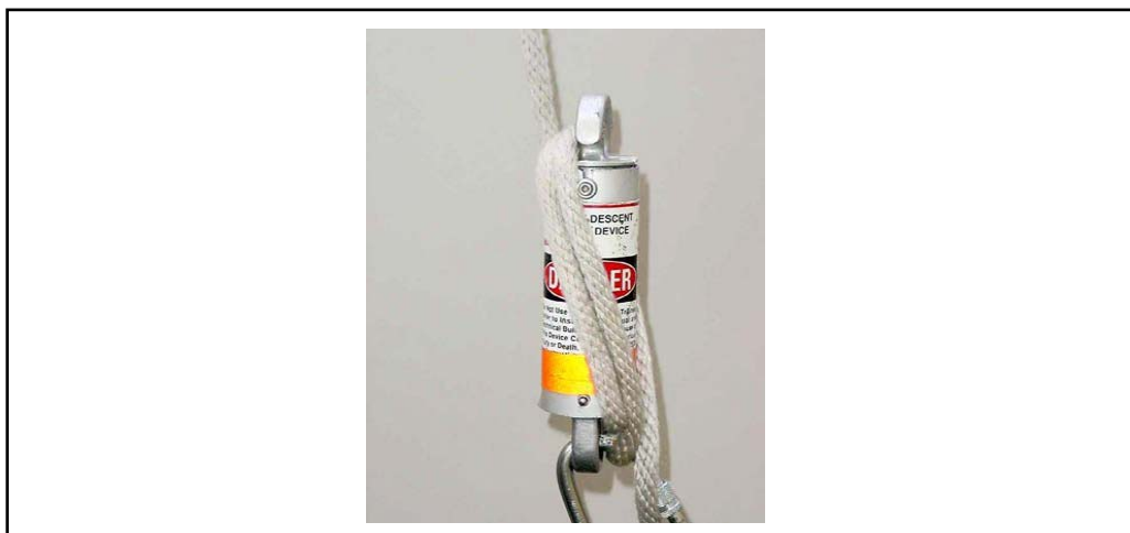
Figure 4-33. Descent Control Device Modified Lock-Off
