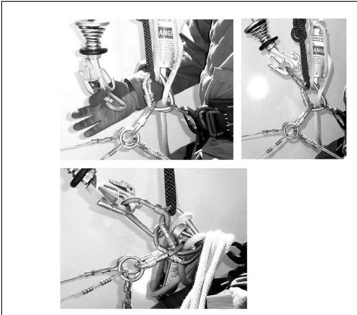
Figure 4-38. Dual-Man In-Flight Hoist Recovery (Rescue/MEDEVAC Litter)
