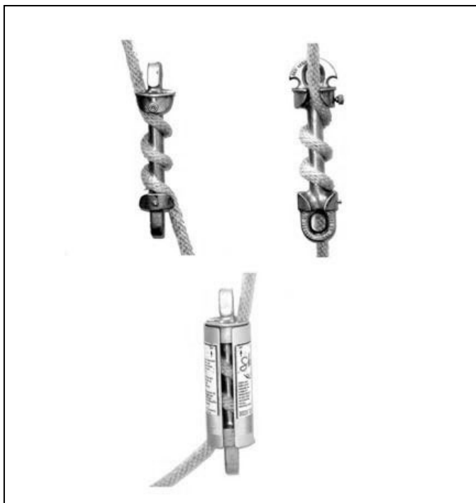
Figure 4-28. Descent Control Device Rigging
