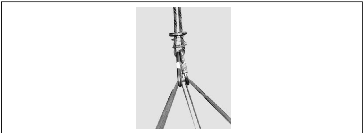
Figure 4-20. Belay Attachment to Cordelette Deck Set-Up
