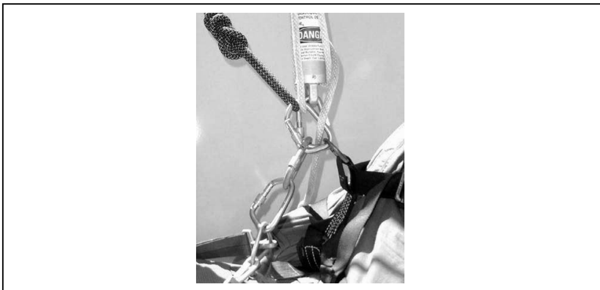
Figure 4-35. RA and Survivor (Hoisting Vest) Short Haul
