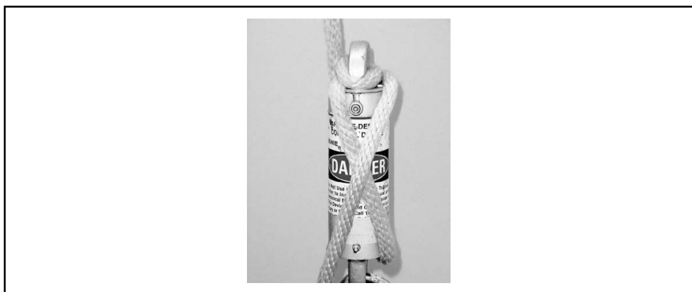
Figure 4-32. Descent Control Device Double Lock-Off
