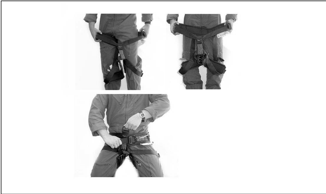
Figure 4-24. Donning the Rappel Harness
