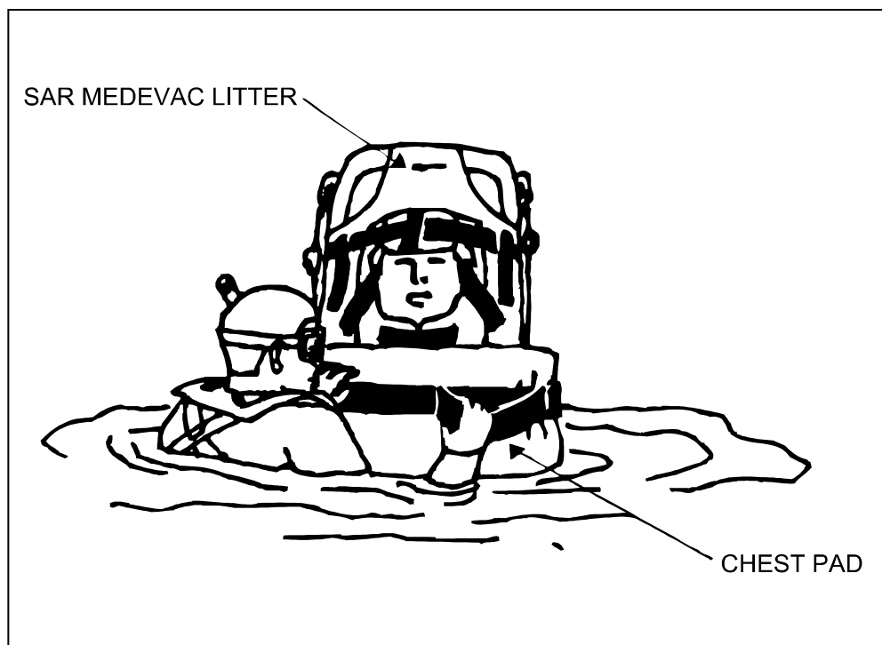
Figure 3-36. RS Secures Rescue/MEDEVAC Litter Chest Pad
