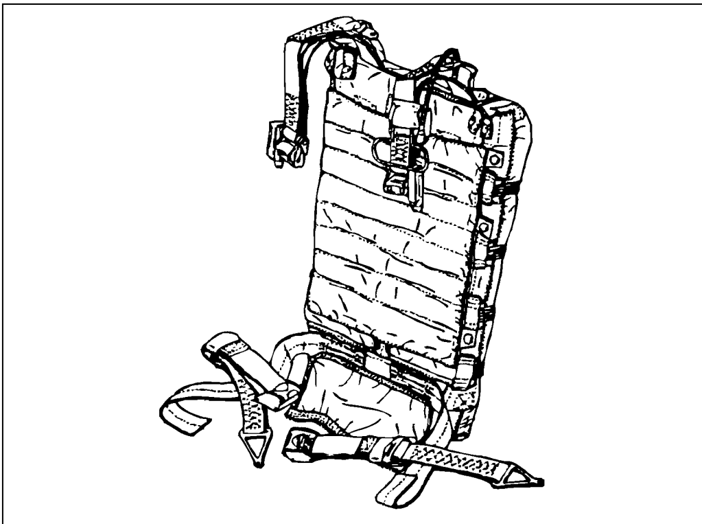
Figure 8-14. NB-7 Personnel Parachute Assembly
