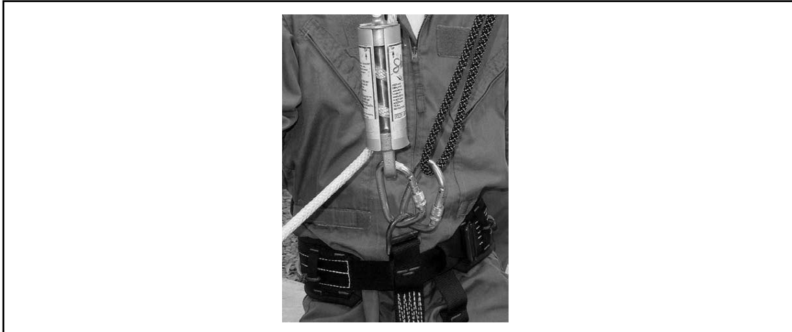
Figure 4-30. Rappel Harness with Both the Descent Control Device and Belay Line Attached
