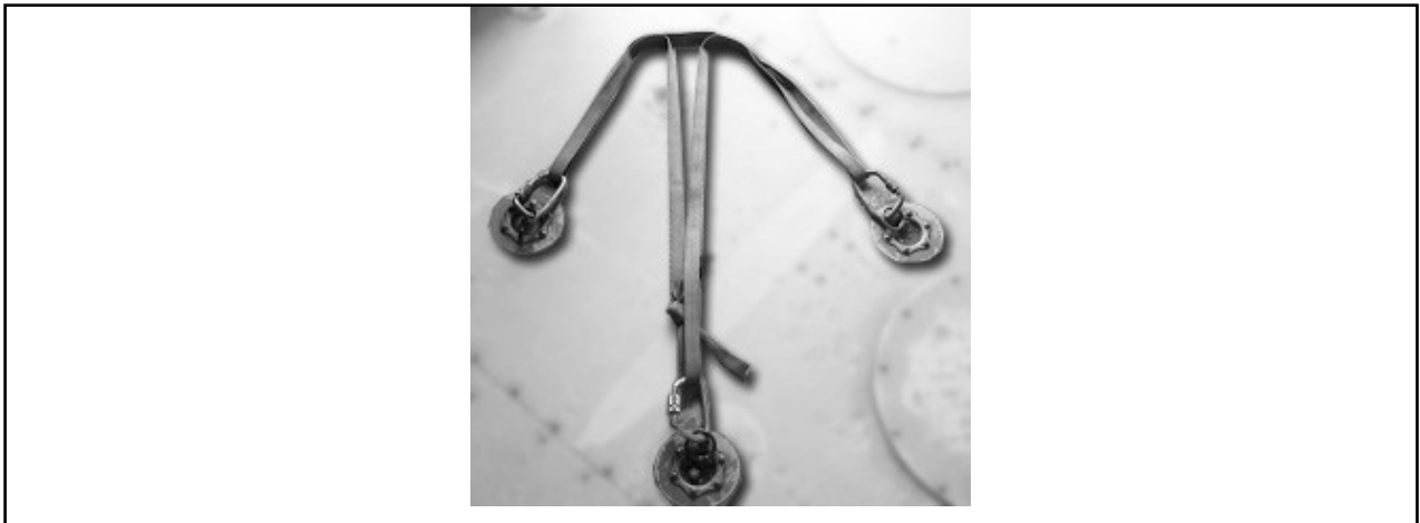
Figure 4-19. "V-Shapes" in Cordelette Deck Set-up
