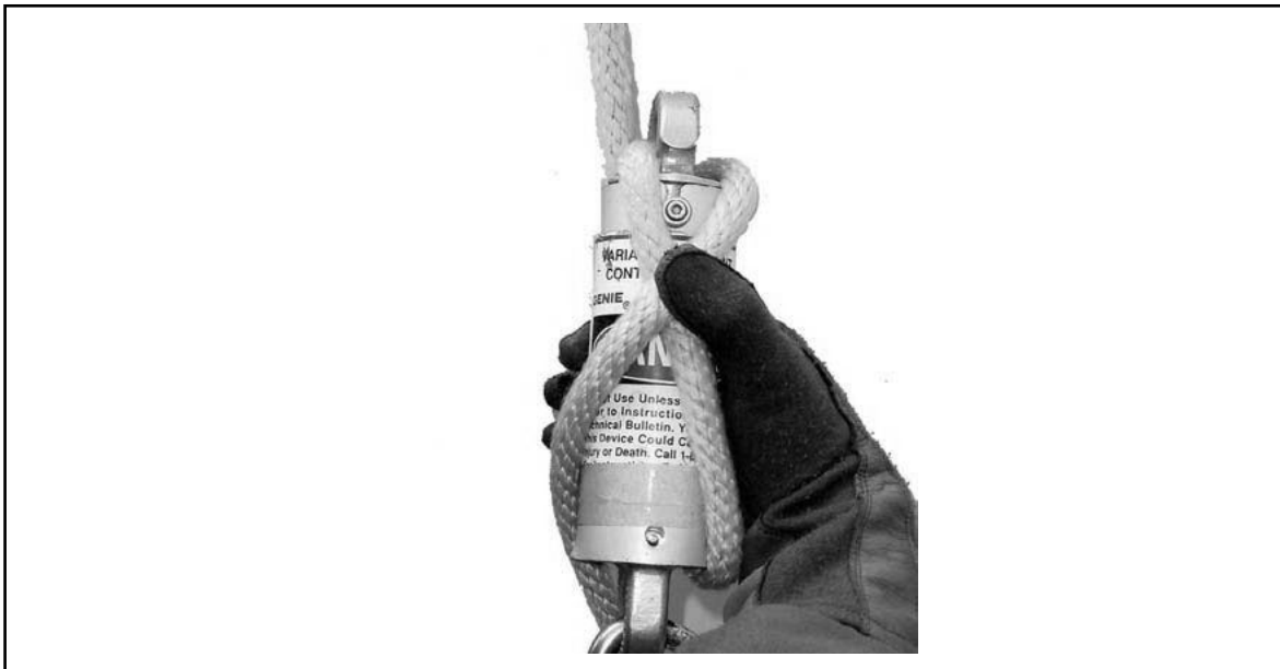
Figure 4-31. Descent Control Device Single Lock-Off
