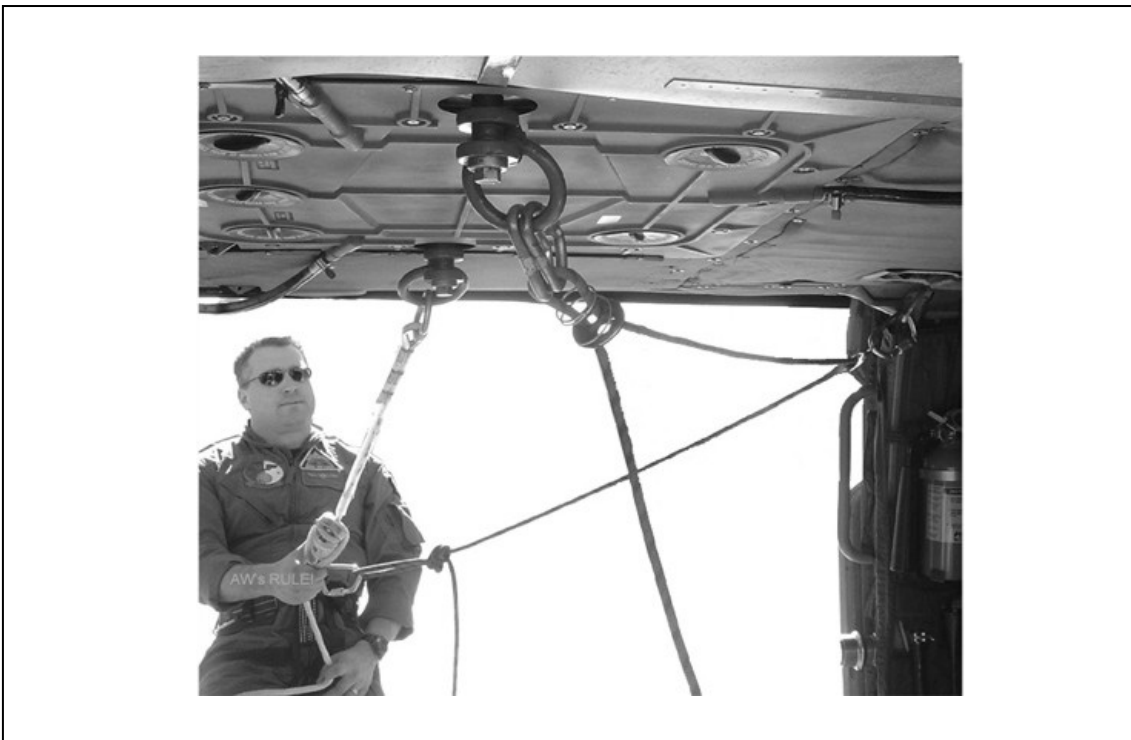
Figure 4-27. H-60 Inland Rappel/Belay Set-Up
